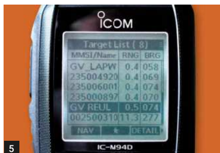
Fig. 1: The new Icom IC-M94DE marine portable VHF with integrated AIS. Fig. 2: The DSC distress button is located under the protective shield on the rear of the transceiver. Fig. 3: The main IC-M94DE display showing selected channel and other information. Fig. 4: The IC-M94DE AIS display. Fig. 5: The IC-M94DE AIS target list display. Fig. 6: The AIS information for a selected 'target'.
